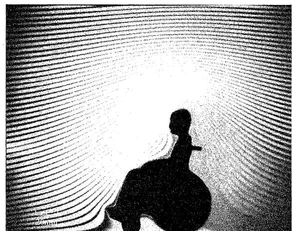
Fig.4 Streamline around wheelchair (No.2)
